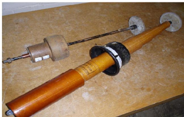
Figure 5.4B – Test Bushings for **Metal Enclosed Switchgear**
