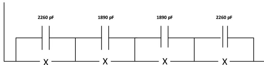
When undertaking invasive GIS works, to ensure that trapped charge is fully dissipated prior to the commencement of work, all **HV Equipment**, associated contacts and conductors to be worked on shall be **Earthed** to ensure adequate dissipation of trapped charge on every part of the **HV Equipment**.
