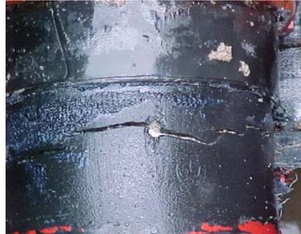
Figure 2: Sheet cracking
