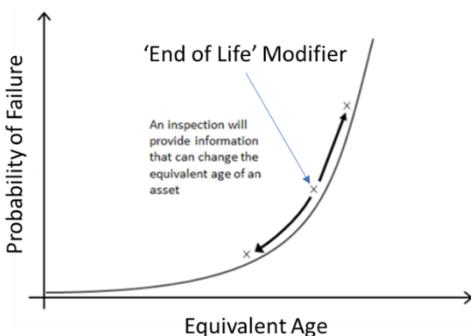
This figure illustrates the principle of the End of Life Modifier. The rise in monetised risk is governed by an asset’s probability of failure plot, the magnitude of the risk at any given point in time is a function of the probability of failure (variable) and the probability of an event with a monetised consequence (fixed).
