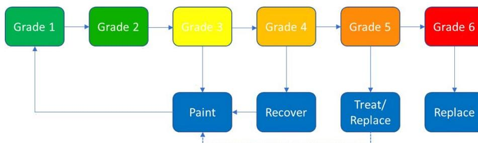
Figure 2. Tower steelwork grade progression
