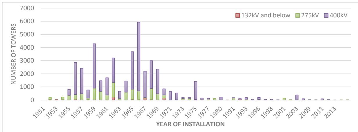
Figure 5: Age profile of overhead line towers
