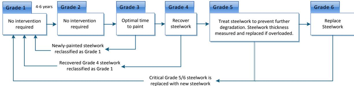
Figure 6. Steel grade and intervention flowchart
