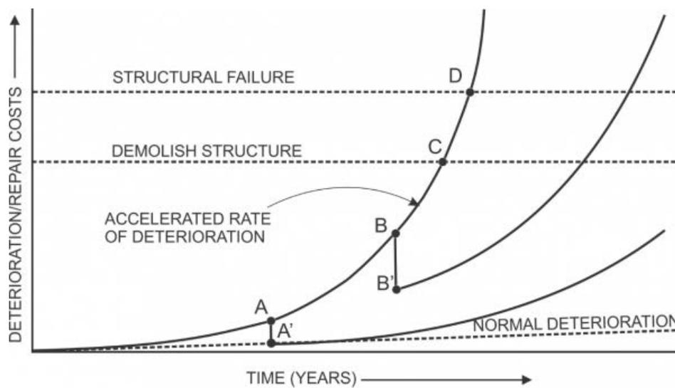
Figure 10. Example of Deterioration Curve aligned with OHL Tower Foundation Performance
