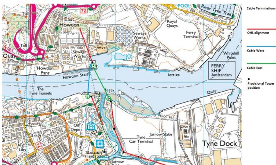
Figure 5: Indicative routes for cable crossing for HDD cable solution
