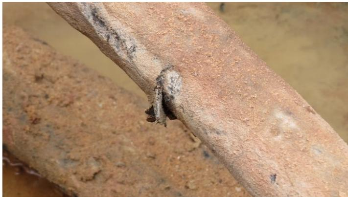
*Figure 5: shows a compromised Hessian outer sheath* [REDACTED]
